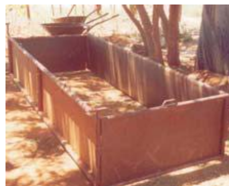
Fig. 2 – Forma montada 3,0 x 1,0 x 0,5m
